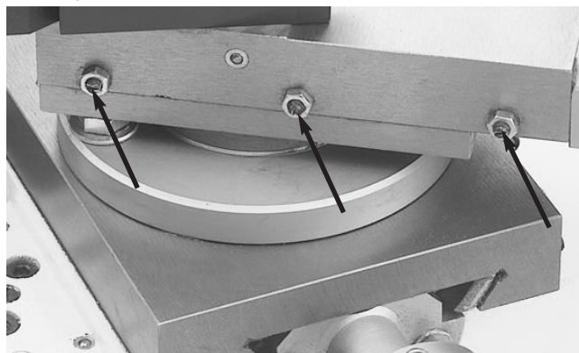
Compound slide gib screws
