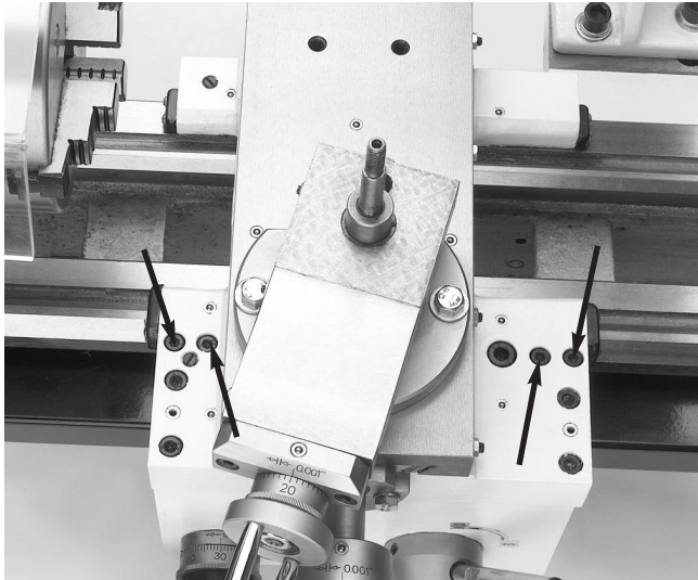
Front saddle gib screws
